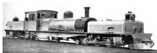
Figure 7: Bayer Garrett narrow gauge locomotive, similar to those on WHR.
